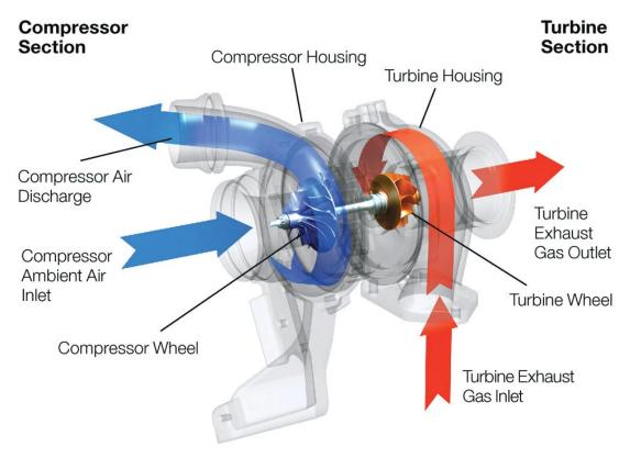
The modern turbo is essentially a small turbine attached to the engine, driven by exhaust gases, that forces more air into the combustion chamber, to deliver more speed. Garrett Motion
