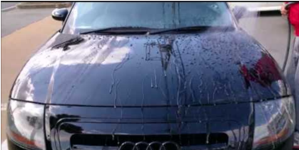
Watch the hydrophobic features on the left side of the car, which is coated vs. right side that's not coated
