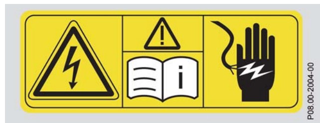
Warning sticker on components of the high-voltage on-board electrical system
