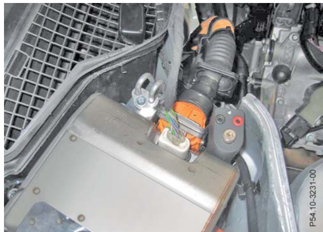
High-voltage battery with high-voltage activation lock installed
