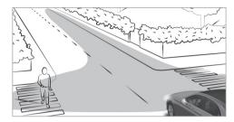
The cornering light improves the illumination of the road over a wide angle in the turning direction, enabling better visibility on tight curves, for example. It can be activated only when the low beam is switched on.
