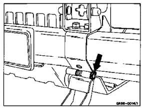
15 Insert quick-release bolts in stop joint.
