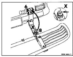
Note: Clearance between impact protection bar and front edge of vehicle should be 20 mm (arrows).
