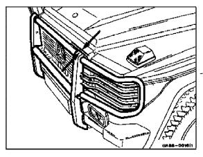
11 Align protection bar left and right by finely adjusting the hinge bolts (8).
