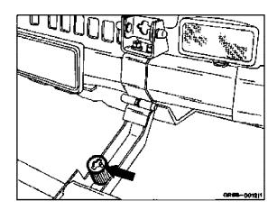
10 Adjust quick-fastener (8) to front end of vehicle by screwing in or out.
