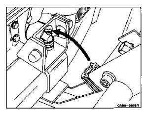
16 Tighten quick-release bolt with enclosed special wrench.
