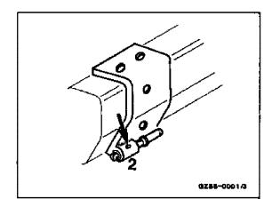
14 Fit impact protection bar. Secure hinge bolts with cotter pins (arrow).
