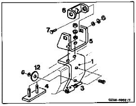
9 Screw quick-fastener into impact protection bar. Slide protection bar onto hinge bolt (5).
