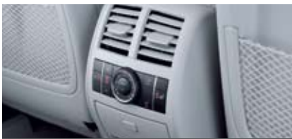
Rear air conditioning
