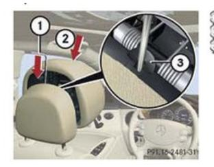
Resetting tool Press back head restraint cushion Guide
