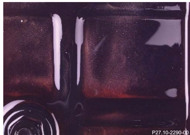
Oil pan with normal wear debris
