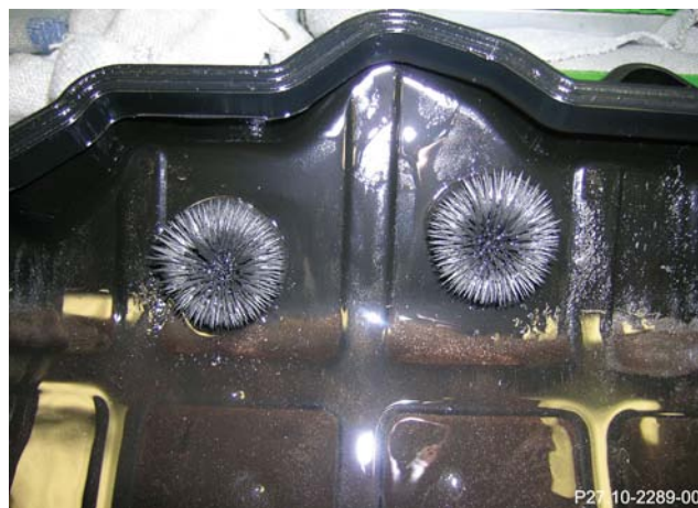
Oil pan with significant wear debris
