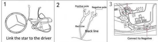
You can also install the LED star badge by replacing the fuse, which can be connected to any control interface according to your needs. For example: car light fuse, unlock fuse, brake light fuse interface, etc.
