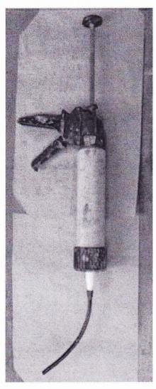
until the cavity between the panels is completely filled. Lead hose through the hole (9) to the skin paneling side panel. Pull out the hole slowly and apply sealing material
