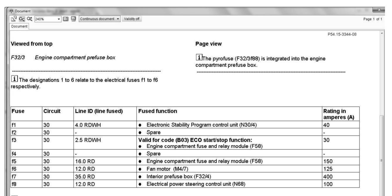
i The electrical fuses f7 and f8 are located inside the plastic housing.
