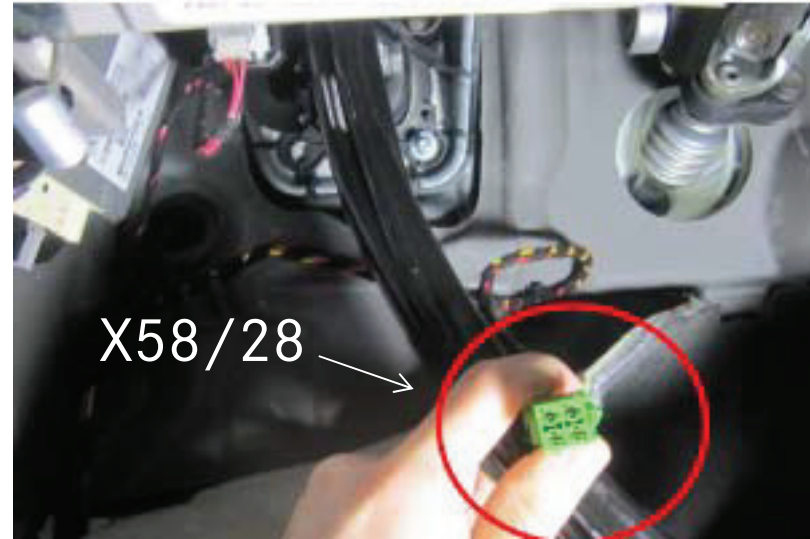
Can be identified by the green connector on the end of the harness
