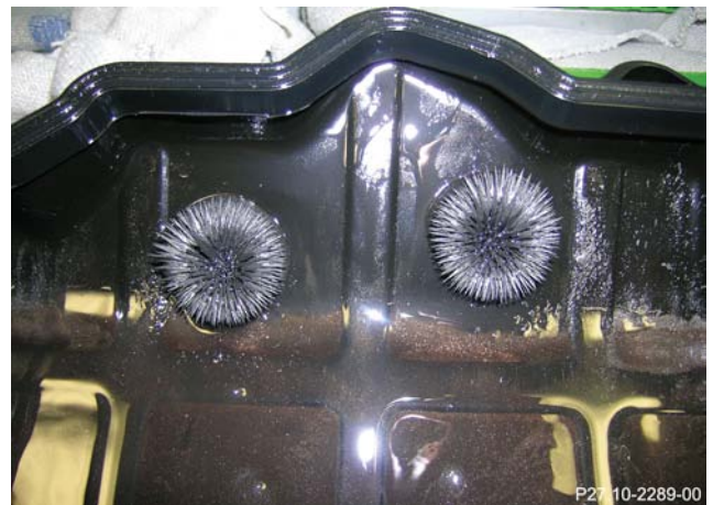
Oil pan with significant wear debris
