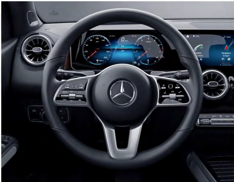
Multifunction Steering Wheel in Leather (L3E) w/ touch control buttons and shift paddles Standard on GLB 250 and GLB 250 4MATIC Not available w/ Steering Wheel Heating (443)
