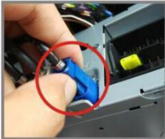
8, Pull out the LVDS connector from original head unit
