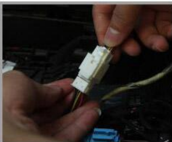
4, Disconnect the cable behind the center console board
