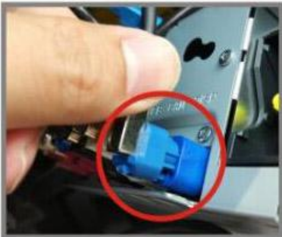
9, Connect Carplay LVDS connector blue side to original head unit
