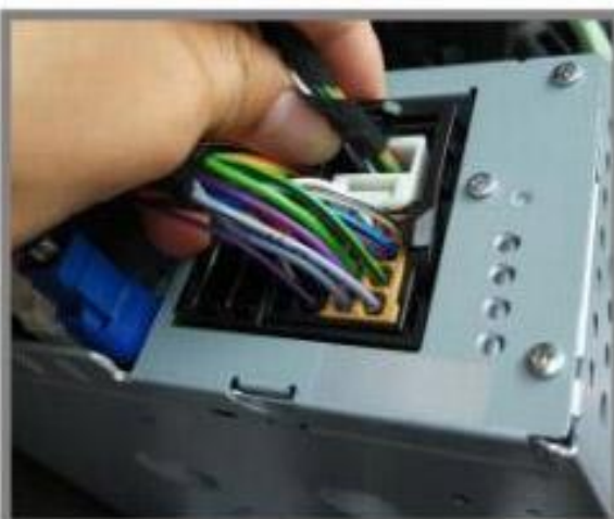
5, Take out original headunit, pull out original RCA connector
