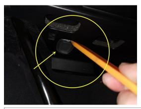
7. Remove the left front foot socket lamp
