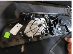
5. Use pliers to remove the aluminum alloy cover of the midrange and fasten it to the midrange bracket with ambient light of this product.
