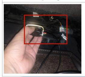
3. Connect the product back light harness to the foot socket light plug under the front seat.
