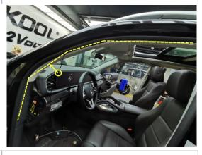
6. Lay the ambient light wiring harness from the B-pillar along the front door frame
