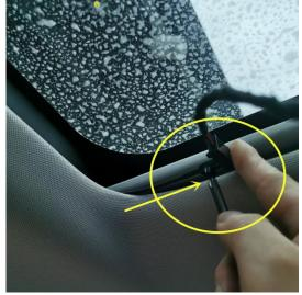
1. Use double-sided adhesive to glue the light guide strip covered with silicone strip to the gap between the sunroof slide rail and the roof on both sides of the car roof
