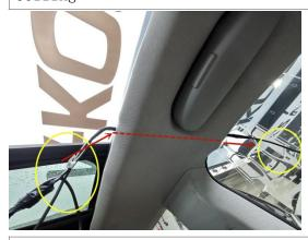
5. Pass the ambient light harness out from above the B-pillar  $\,$
