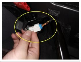
8. Adapter the sunroof atmosphere light harness plug to the left front foot socket light plug for power
