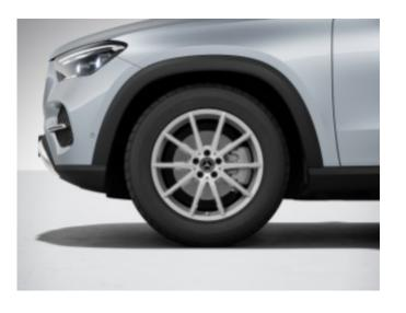
27R - 19" 10-Spoke Wheels For GLE450E4, Extended Mobility Tires (R66) replaces spare wheel (690) 19" R02 (All-Season tires), 690 (Spare Wheel) 19" Twin 5-Spoke Wheels 255/50 R19 on 8 J x 19 ET 61 (Front) 255/50 R19 on 8 J x 19 ET 61 (Rear)
