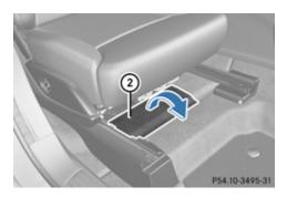
Fold the piece of cut carpet 2 in the direction of the arrow.
