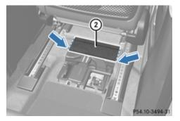
Use a sharp knife on carpet 2 to cut along the dashed white line until you reach the perforated part. Position the right-hand front seat at its rearmost position.
