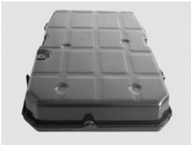
Figure 1. Oil pan (with round forms) transmissions 722.9 up to production date June 21, 2010 P00-40-2027-01
