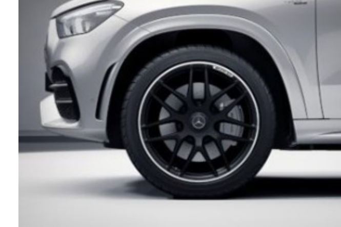
RXV - 22" AMG Cross-Spoke Forged Wheels, Matte Black 22" R01, 669 AMG Cross-Spoke Wheel, Matte Black 285/40 R 22 on 10 J x 22 ET56 (Front) 325/35 R 22 on 11 J x 22 ET52 (Rear)
