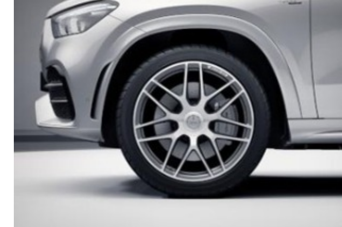
RXU - 22" AMG Cross-Spoke Forged Wheels 22" R01, 669 AMG Cross-Spoke Wheel 285/40 R 22 on 10 J x 22 ET55 (Front) 325/35 R 22 on 11 J x 22 ET53 (Rear)
