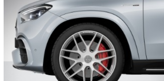
RXU - 22" AMG Cross-Spoke Forged Wheels 22" R01, 669 AMG Cross-Spoke Wheel 285/40 R 22 on 10 J x 22 ET55 (Front) 325/35 R 22 on 11 J x 22 ET53 (Rear)
