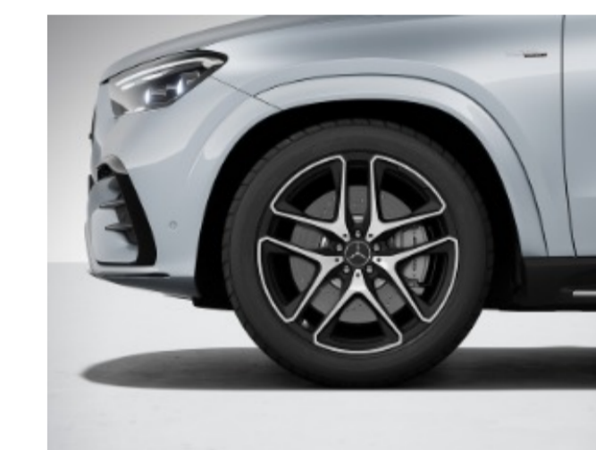
RWE - 21" AMG Twin 5-Spoke Wheels w/ Black Accents only icw AMG Night Package (DC1) 21" R02, 669 AMG Twin 5-Spoke Wheel, Matte Black 275/45 R 21 on 10 J x 21 ET51 (Front) 315/40 R 21 on 11 J x 21 ET47 (Rear)
