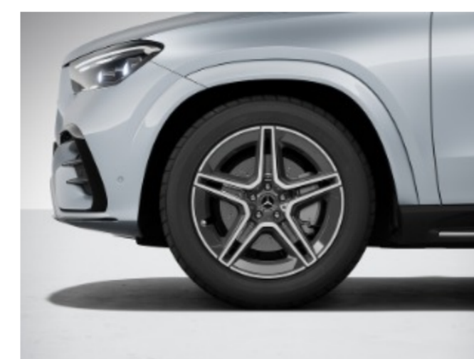
RZV - 20" AMG 5-Spoke Wheels Standard on GLE 53 20" R01, 669 AMG Twin 5-Spoke Wheels 275/50 R20 on 9 J x 20 ET 57 (Front) 275/50 R20 on 9 J x 20 ET 44 (Rear)
