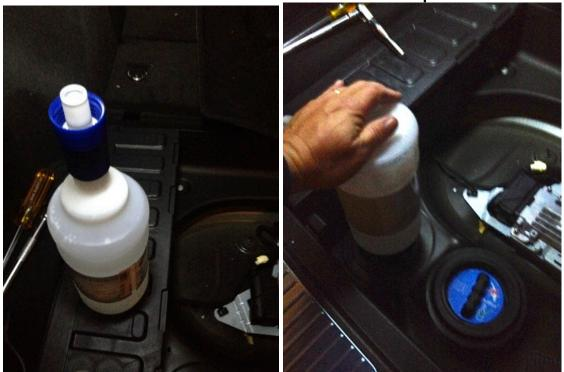
5. **Press downward on the bottle to release the ADBLUE into the tank**. The bottle feels like it is spring loaded, and will move down about an inch. Note: there is a tube inside the bottle that enables air to escape the tank while the bottle is emptied. This bottle will be re-used as the funnel when the larger DEF bottles are used to fill the remainder of the tank.
