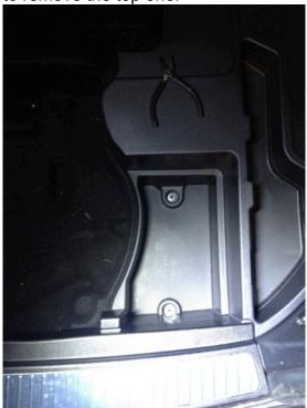
3. Once the nuts are removed, **gently pull up on the plastic cover that was held down by the nuts, while pulling the molded storage cover up and forward**. It can be wiggled out with a little effort. Once the cover is removed, the cover to the ADBLUE fill port will be clearly visible in the lower left. **Twist and remove this outer cover to expose the actual fill port cover**.
