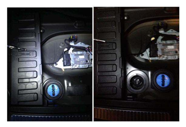
4. **Unscrew the tethered fill port cover** and move it aside. Unscrew the top of the half gallon ADBLUE bottle. **Invert the bottle and screw it onto the fill port**.
