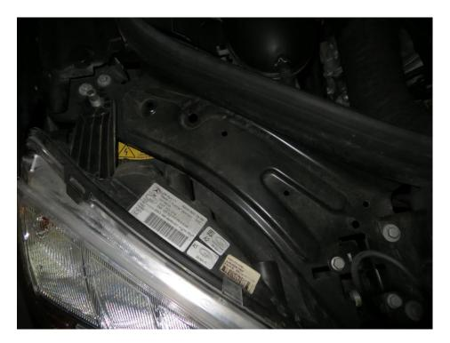
The black knob that holds the bulb for the front marker light is at the top outside corner of engine bay. Turn this knob counter-clockwise and pull the knob out.
