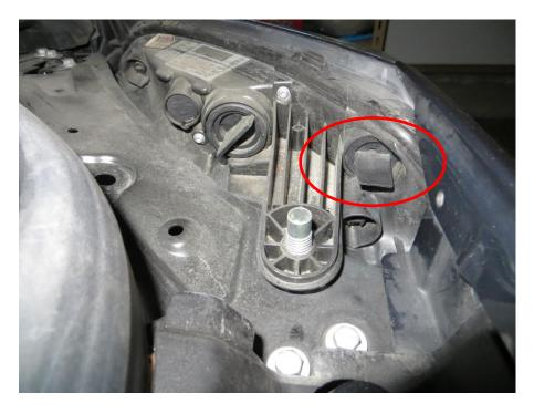
The knob has the bulb at the other end of the knob. Pull the bulb straight out and replace with new bulb.
