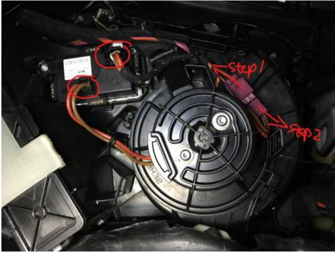
Next gently pull down on the tab on the side of the blower motor (red arrow). With the tab pulled down turn the motor clockwise and wiggle and pull it down and out of the housing.
