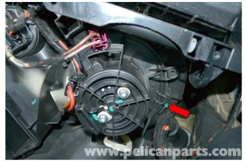
With the motor out of the vehicle you can better see the tab you will be gently pulling down on (red arrow).
