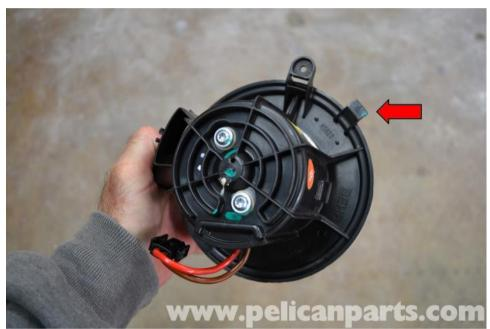
The housing goes up to the air box in the engine compartment (red arrow). Make sure to clean the housing, as all kinds of things can get in there.
