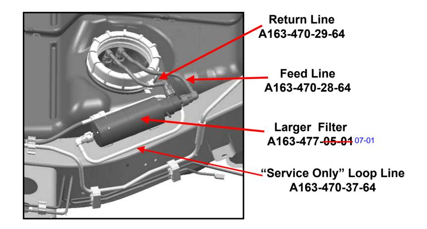
The larger filter is installed in production as of approx. March 26, 2001 and does not require the "service only" loop line.
