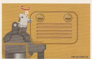
The manual release is located behind the cover in the left rear compartment trim panel.
