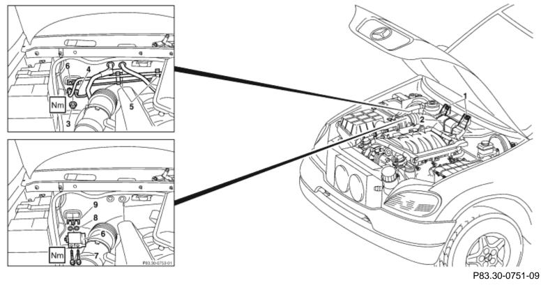
1 Expansion reservoir nut 2 Expansion reservoir 3 Self-locking nut
