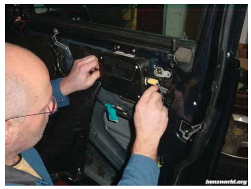
replace the cable in the original postion by feeding it back underneath the airbag!
