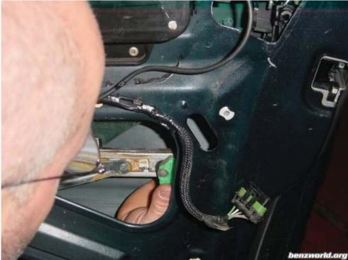
NOTE: As said earlier don't screw the lock in place until you have the guide rail in position.
