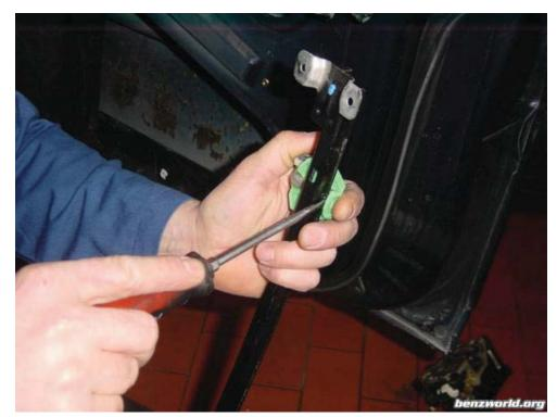
You can either unclip the lift connector , or unscrew the lock again! We chose to unscrew the lock as it was a lot easier to manouver the rail in place!
