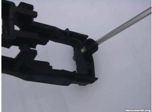
Note the screw for the outside door handle end piece.
