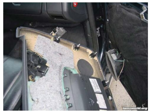
push the panel back into place. Best to hook the top in place first (over the door pin), then let it hang there while postioning the white clips correctly at the bottom.
