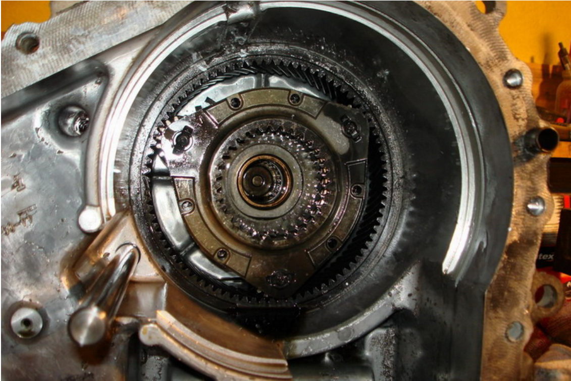
9. Remove Low/High speed Planetary Carrier (expand snap ring)
