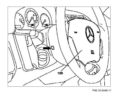
After removing bolt make mark on shaft and steer. wheel
