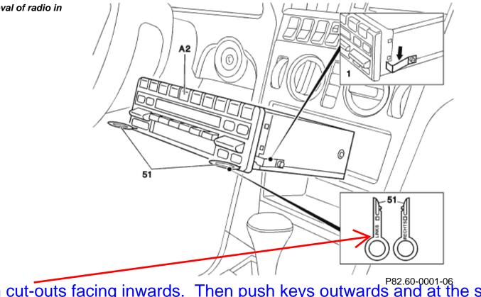
Insert keys with cut-outs facing inwards. Then push keys outwards and at the same time pull radio out.
