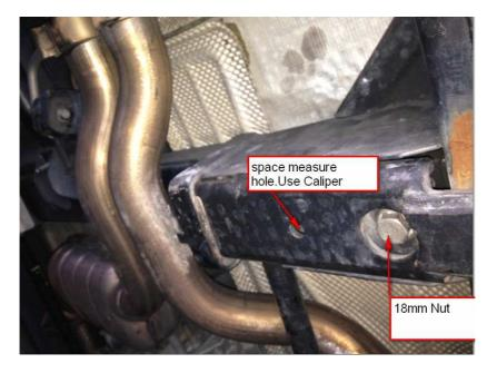
2. Using the caliper to measure the current gape (mine shows 43mm)
