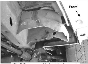
(Fig 5) Passenger side front body mount pictured after plastic cover removed
