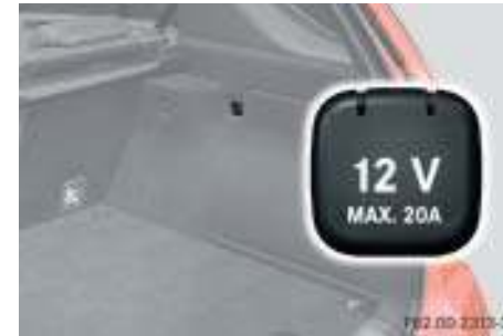
Power outlet in cargo compartment
