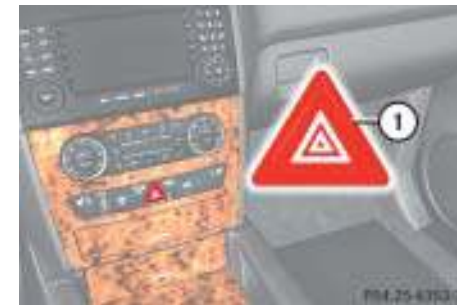
① Hazard warning flasher switch
