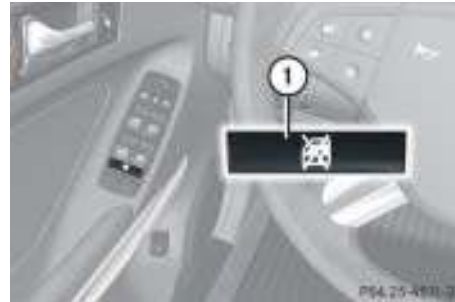
① Override switch
