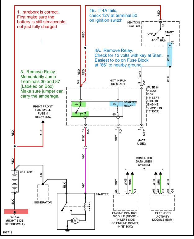
2. Not likely the cause, but check for 0 ohms from battery negative to another point on chassis
