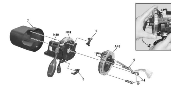
4 Bolts 5 Cover 6 Cover 7 Steering column switch module paneling
