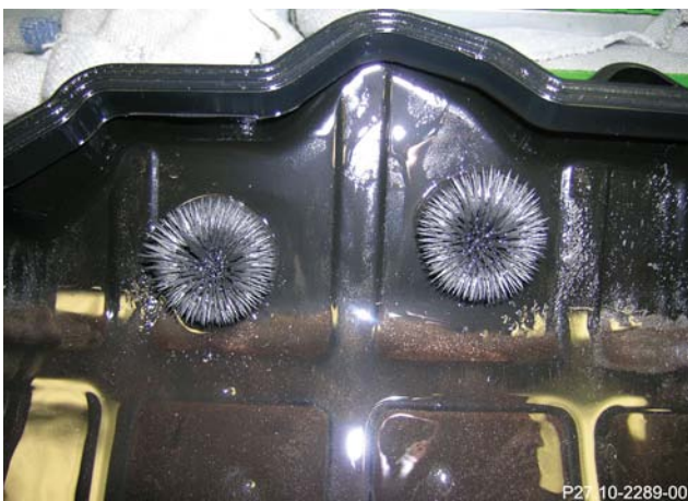
Oil pan with significant wear debris
