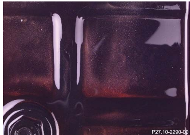
Oil pan with normal wear debris
