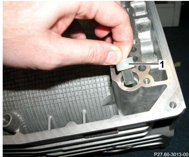
1 Converter return flow strainer Electrohydraulic controller unit removed, front of transmission housing, on left in direction of travel
