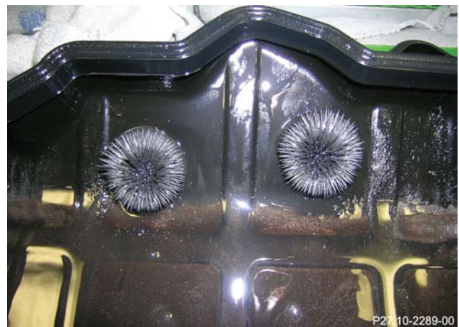
Oil pan with significant wear debris
