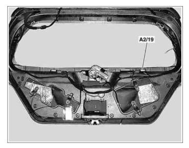
The FM rear window amplifier is decoupled from the vehicle
