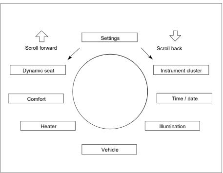
Press the system selection button (S110s3) until the menu "Settings...Reset: Press reset button for 3 seconds" appears in the multifunction display (A1p13). Go to the menu point settings with the scroll forward and backward buttons (S110s1) (↑).
