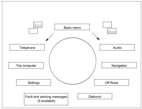
The above system selection illustration shows the possible systems on a circle. Each time the driver presses the system select/voice control pushbutton (S110s3) the display jumps to the next system.
