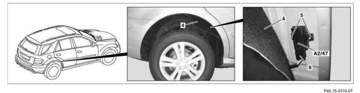
4 Panel in right rear fender liner5 Nuts
