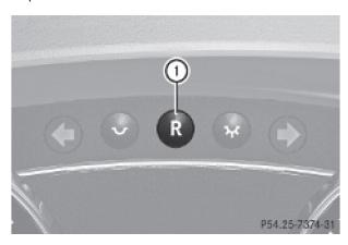
➤ Clearing the maintenance service indicator message manually: Press reset button ① on the instrument cluster.
