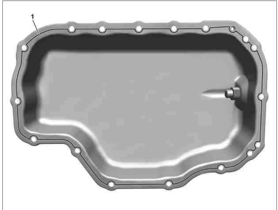
Oil pan bottom section for engine with front sump without code M005
