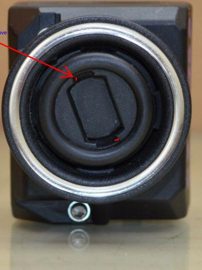
use needle nose pliers to remove ring if you do not have tool
