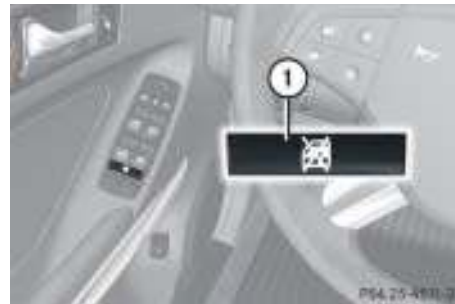
① Override switch
