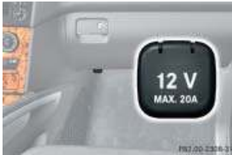
Power outlet in front passenger footwell
