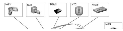
A1 Instrument cluster B38/2 Rain/light sensor M5/1 Windshield washer fluid pump M5/2 HCS pump M6/1 Wiper motor M6/4 Tailgate wiper motor M14/5 Right front door CL motor M14/6 Left front door CL motor N10 Front SAM ECU N10/8 Rear SAM control unit N70 Overhead control panel control unit N73 EIS control unit N80 Steering column module N93 Central gateway control unit S4 Combination switch
