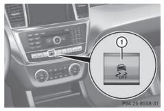
▶ To deactivate: press button (1). The [基] ESP® OFF warning lamp in the instrument cluster lights up.
