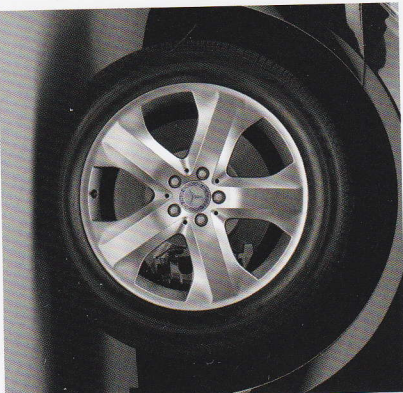
19-inch 5-spoke light-alloy wheel with mixed-size tyres (optional)
