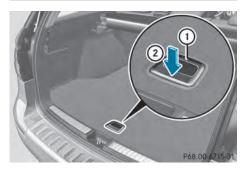
A removable insert under the cargo compartment floor contains the parts of the EASY-PACK load-securing kit. The tirechange tool kit is stored beneath this insert.
