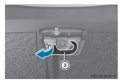
► Fold out hook ③ on the underside of the cargo compartment floor in the direction of the arrow.
