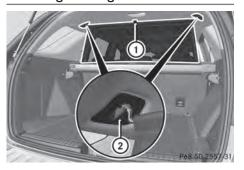
▶ Pull the cargo net up by tab ① and hook it into eyelets ② using both hands.
