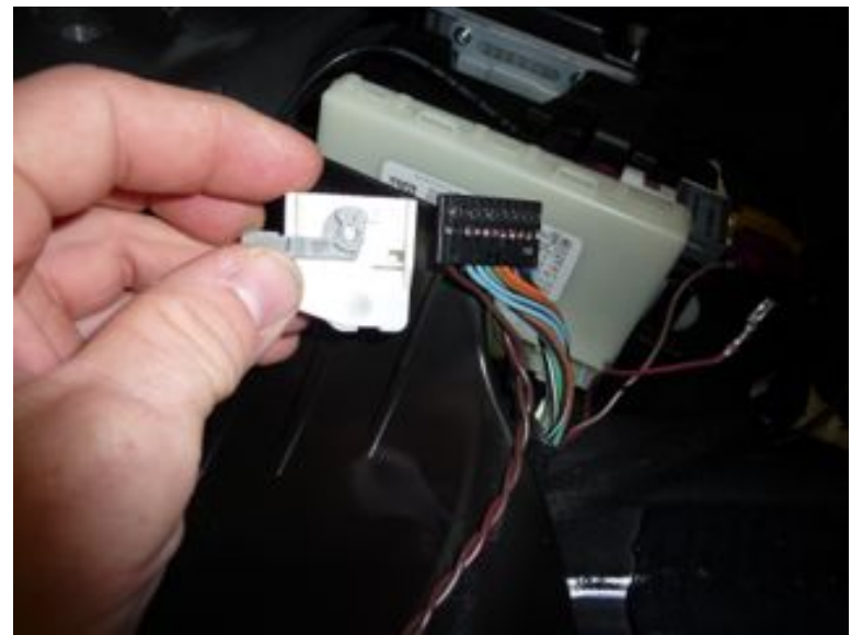
New pins installed, reinstall shroud
