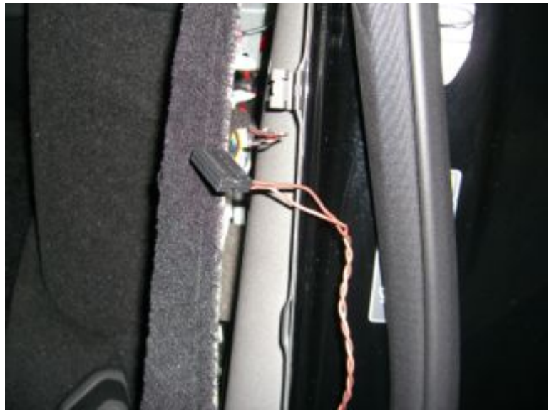
KG harness properly installed into plug
