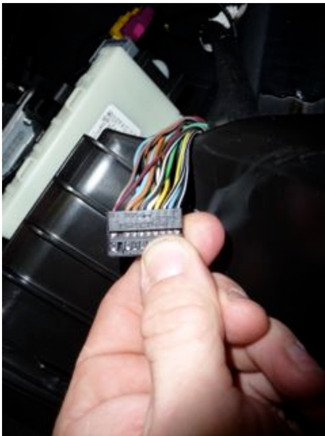
Shroud removed from plug
